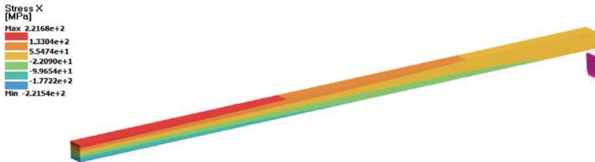
Figure 15: SimSolid – Direction stress acting in a direction parallel to the length of the beam
